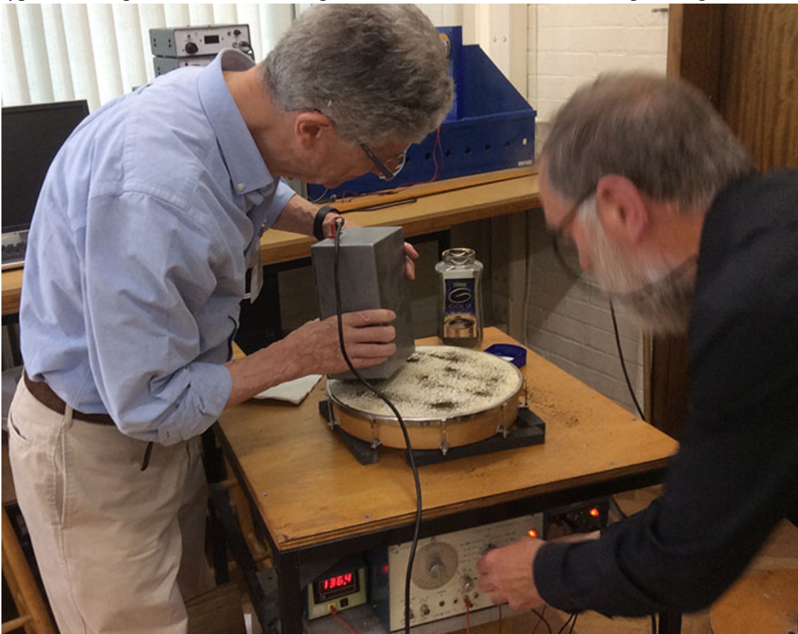
The author and Professor Woodhouse experimenting with the Chladni method in Cambridge Engineering Department. Photograph: courtesy David Hyams
